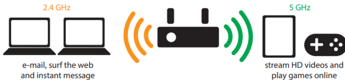
Figure 2: Wi-Fi dual-band technology [17]
