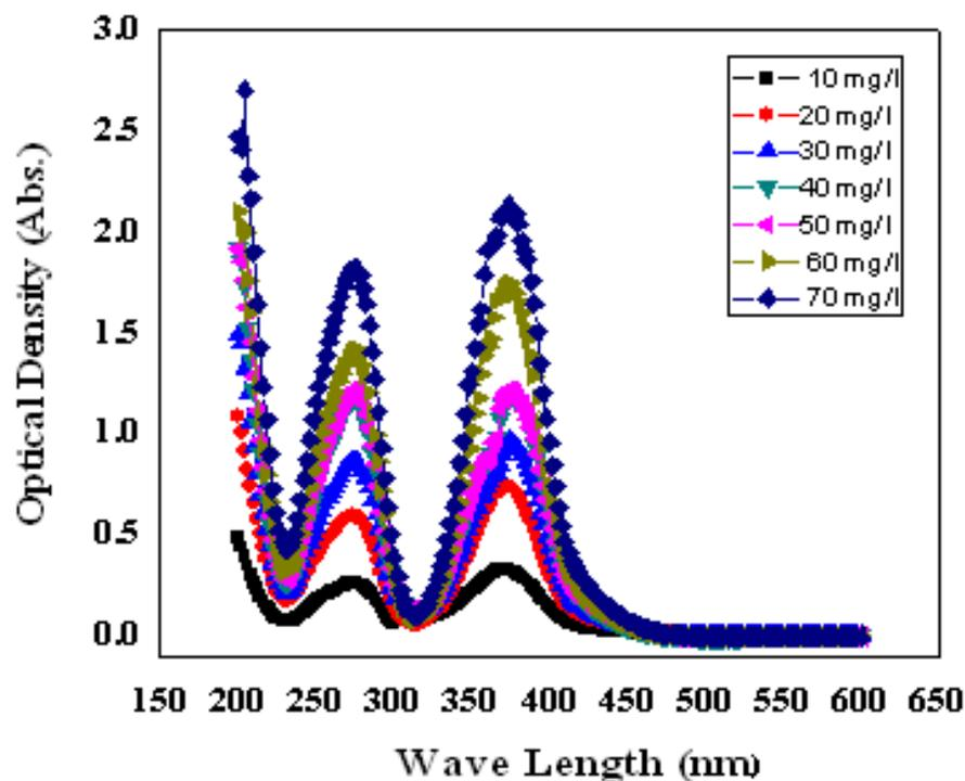
**Figure 1:** UV-visible spectra of 7 standard Cr(VI) aqueous solutions at pH=7
