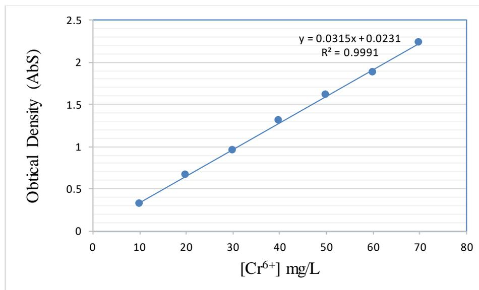
**Figure 2:** Calibration curve in Cr(VI) aqueous solutions at  $\lambda = 373$  nm.
