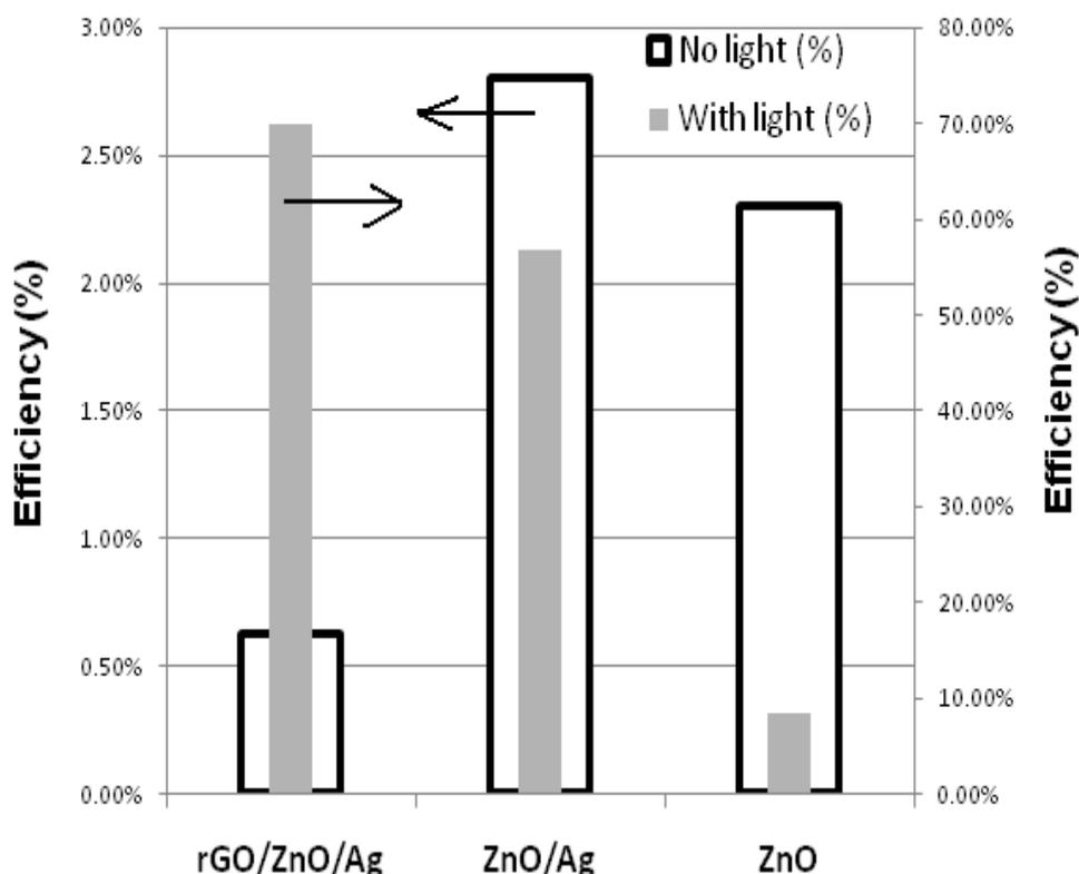
**Figure 8:** Values of efficiency for photocatalytic reduction of Cr(VI) to Cr(III) when used ZnO, ZnO/Ag and rGO/ZnO/Ag as nanocatalysts, with or without UV light irradiation. (Initial Cr(VI): 50 mg/L at pH 7)
