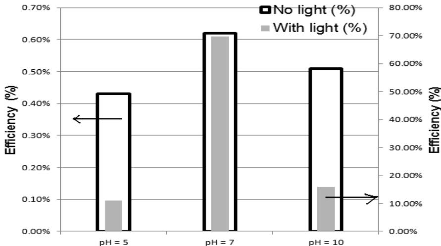
**Figure 9:** Effect of pH on the efficiency for photocatalytic reduction of Cr(VI) to Cr(III) for rGO/ZnO/Ag as nanocatalysts, with or without UV light irradiation. (Initial Cr(VI): 50 mg/L)
