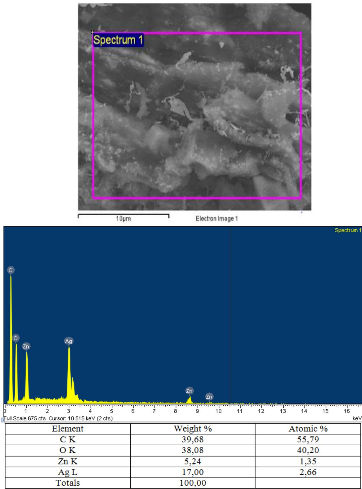
Figure 6: EDX result of rGO/ZnO-Ag nanohybrid (sample area: 15×20 µm)
