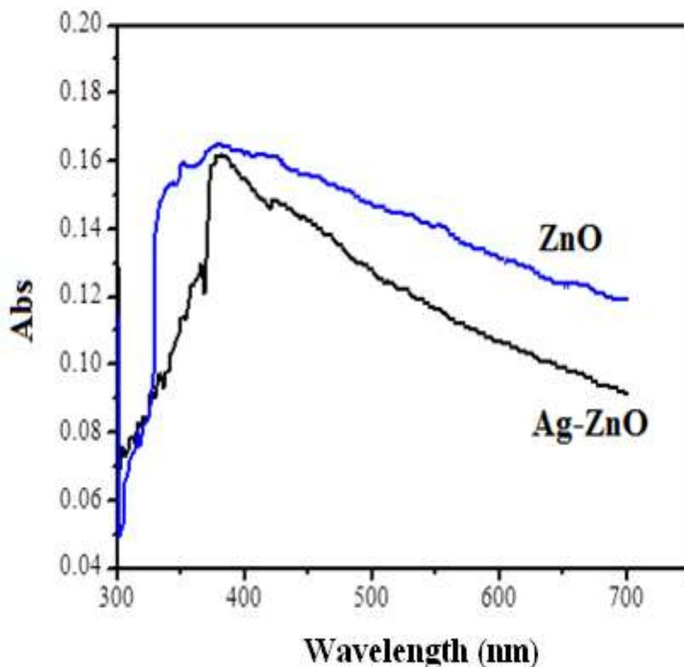
**Figure 7:** UV-visible spectra of ZnO NP and Ag/ZnO nanohybrids dispersed in water
