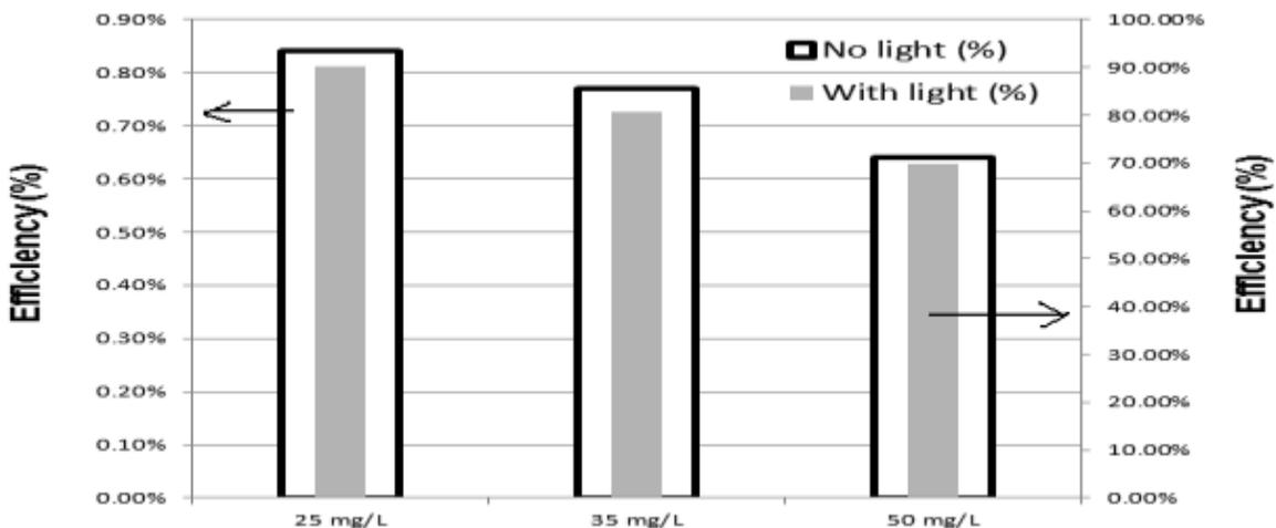
**Figure 10:** Effect of initial Cr(VI) concentration on the efficiency for photocatalytic reduction of Cr(VI) to Cr(III) for rGO/ZnO/Ag as nanocatalysts, with or without UV light irradiation. (pH =7)
